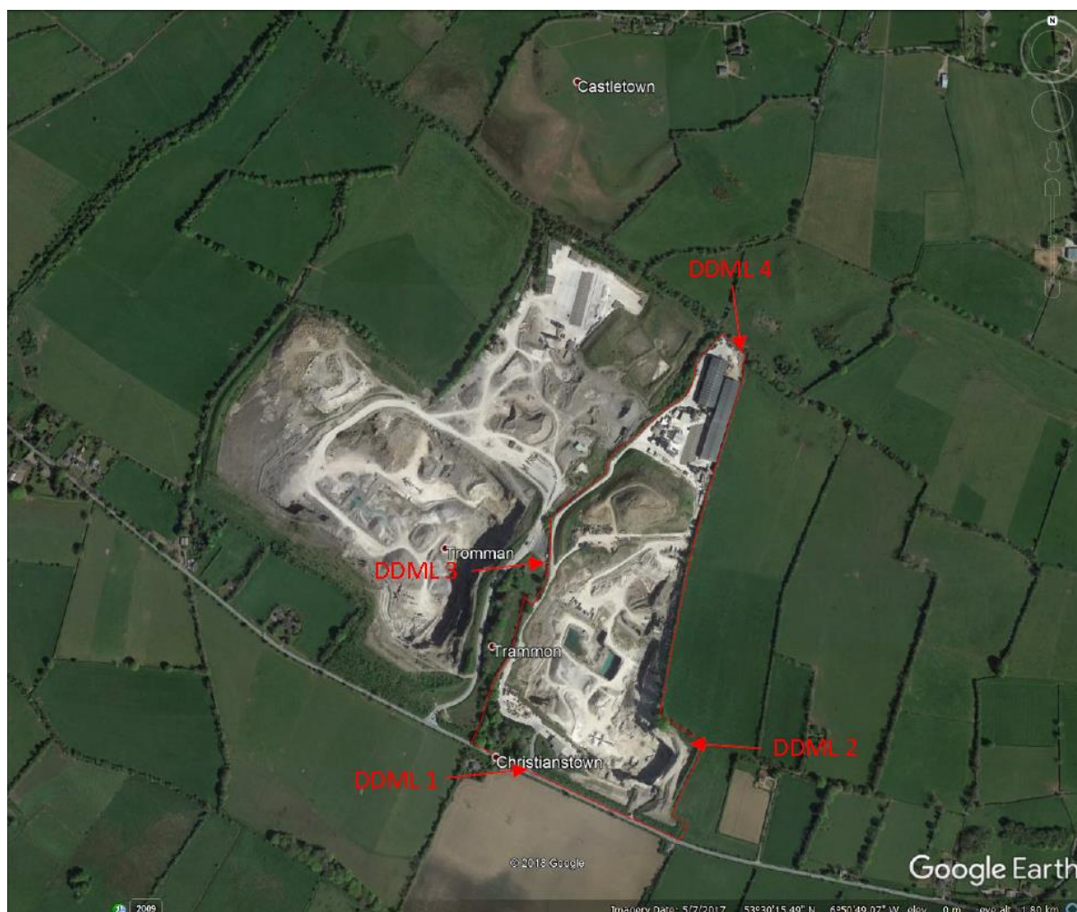
Figure 7.1: Dust deposition monitoring locations (DDML).
